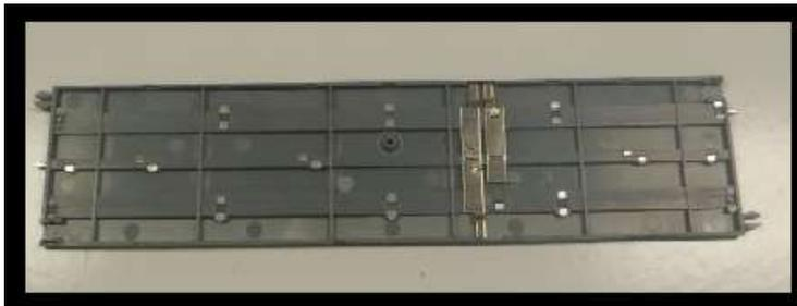
The 2 tracks above are original. This single rack above has a section removed from the outer track connector to isolate the rails.
