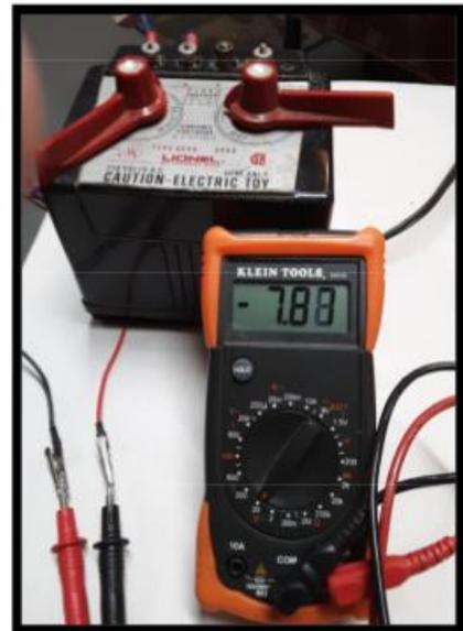
24. Set the power level on the AC transformer to level that is needed and you are ready to test/run any DC motor or other DC device. Adjust the AC transformer power level as needed for different DC equipment.
