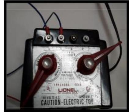
18. Use your variable control or speed control hookup to control the power level to the rectifier.
