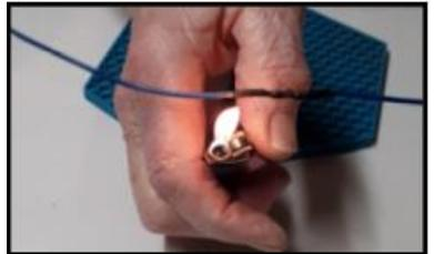
16. If Step 4 is skipped or forgotten and Heat Shrink can't be slid over an open end of the joined wire, use Liquid Tape.
