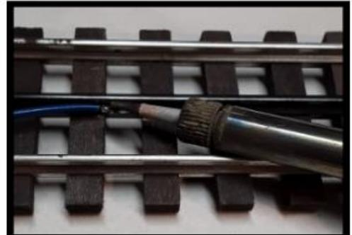
9. Hold wire in place for a few seconds until the solder cools and the wire is attached.
