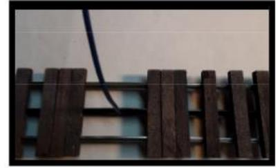
8. Use soldering iron with the heat level turned to high about 30 to 40 watts.
