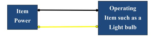
A simple circuit is nothing more than electric power being supplied by some means to operate any electrical item such as a light bulb
