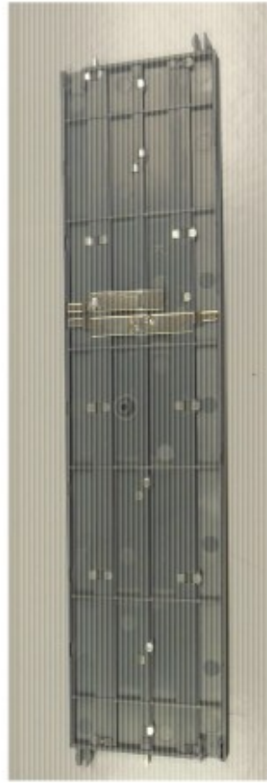
Track above has a section removed from the outer track connector to isolate the rails.
