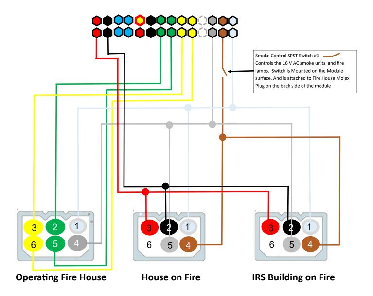
All of the wiring is under the Module with the three plugs mounted on the back side board of the Module itself.
