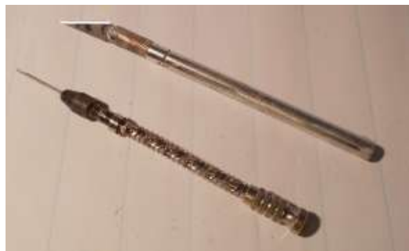
Figure 3: Pin vise drill and X-Acto knife with a #11 blade are both just about indispensable for many projects.
