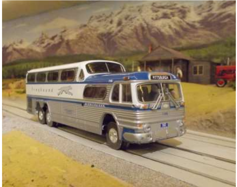
Figure 18: This Corgi 1:50 Greyhound Scenicruiser is a handsome model of this most iconic 1950s cross-country bus, and makes a wonderful conversion. The dual rear axle permits the use of a swiveling truck at the back which makes the bus run well through curves.
