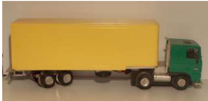
Figure 12: This converted Joel 1:50 model of a DAF KF420 tractor has a medium-size motor (middle, Figure 6) mounted vertically and driving the tractor's front axle. It uses a metal track-speeder chassis and lead shot for weight. The tractor weights a full pound with 12 ounces of it on the front axle. The trailer weighs only 6 ounces. Despite this, it will climb no more than a 4% slope, slows very noticeably on D-21 curves, and barely makes it through D-16 curves. It also exhibits just a trace of the shaking discussed at the bottom of this page.
