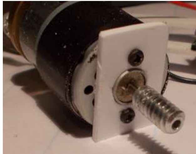
Figure 16: Motor faceplate, installed.
