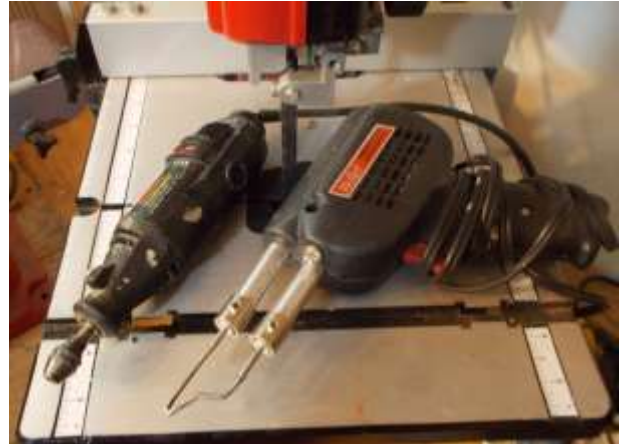
Figure 8: Dremel rotary tool and Weller 260/200-watt solder gun are power tools used quite often in projects covered here.
