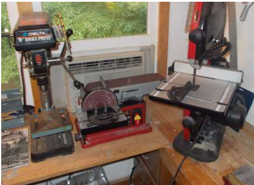
Figure 10: Bench band saw, belt sander, and drill press together cost less than two 'Streets RTR sets but are so very useful. While it is possible to do all projects in this book with handheld tools, these three make work faster and more precise. The author thinks that when these tools are used safely, there is slightly less risk of injury and damage to models than would be the case if he were using only manual tools.
