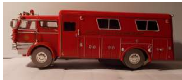
Figure 7: Converted fire truck after five-minute test run. It sits too low at the rear by nearly 1/8 inch.
