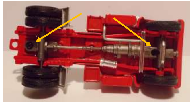
Figure 22: Tractor comes apart once two screws are removed
