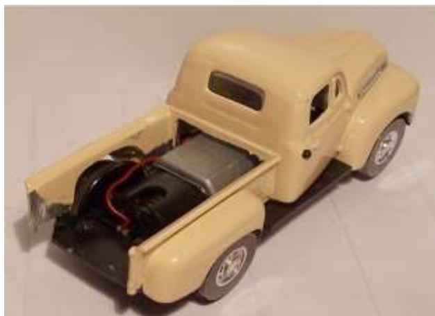
Figure 45: Bed floor is cut out along with spaces for the motor (back of the cab) and wheels (sides of bed), too. That is all the cutting of metal that must be done, period.
