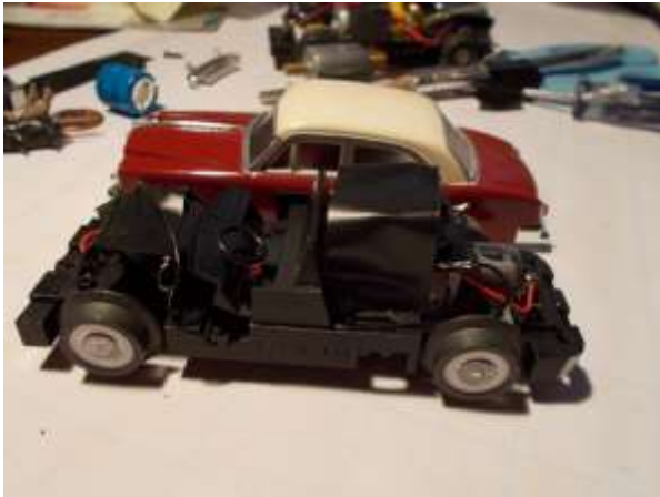
Figure 16: Two supercapacitors are taped in a stack above the motor, and the third above the front axle. The WBB sedan body can accommodate them along with its interior. Some die-cast conversions cannot, and the interior has to be removed to make room for the supercapacitors.
