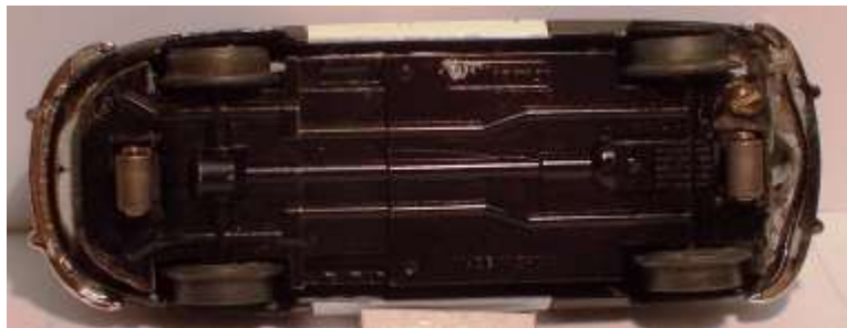
Figure 22: 1950 Nash required chassis corners be rounded and that it be shortened by 3/16 inch up front.
