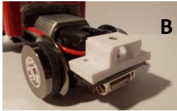
Figure 9: Scratch-built styrene trailer mounting platform is screwed on from beneath.
