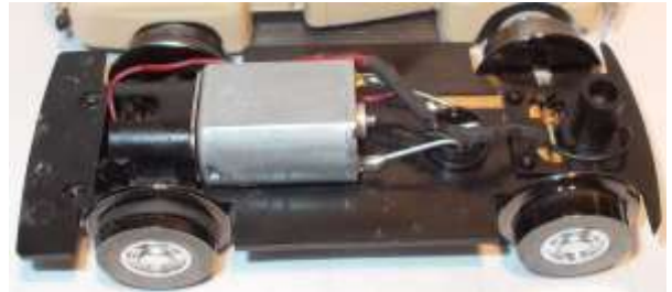
Figure 1: This plastic panel van chassis is laid out like the metal sedan chassis but weighs only a sixth as much and its wheelbase is not adjustable without modification. The step-van, vintage truck, and shorty bus have a plastic chassis, but with different wheelbases and wheel sizes.
