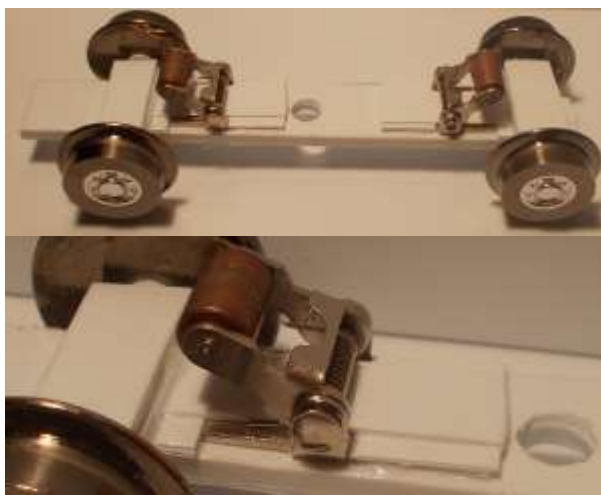
Figure 18: Front and rear center pickups are attached (without wire leads) being held in by plastic sheet plastic welded in place.
