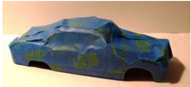
Figure 8: Blue painters tape protects the body during cutting and other operations.
