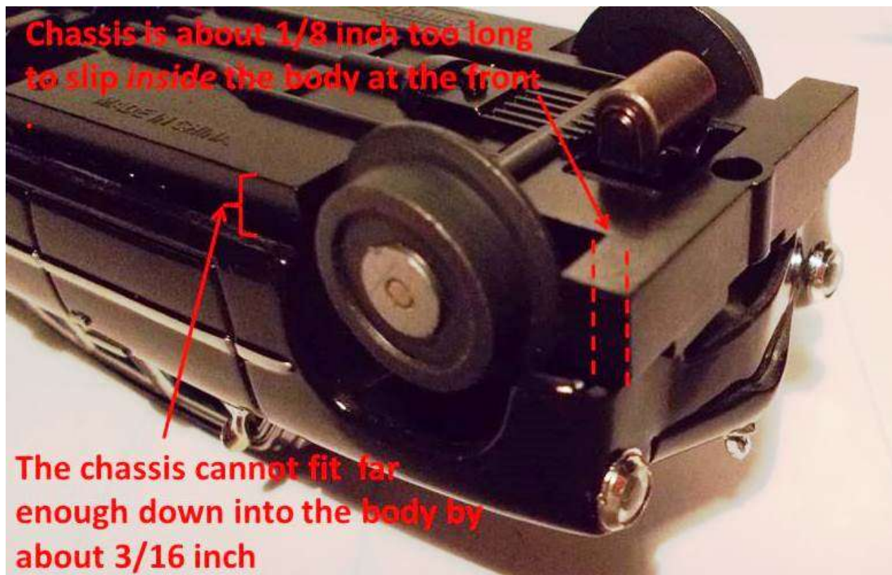
Figure 5: Issues that have to be dealt with to make a good fit. See text for details.
