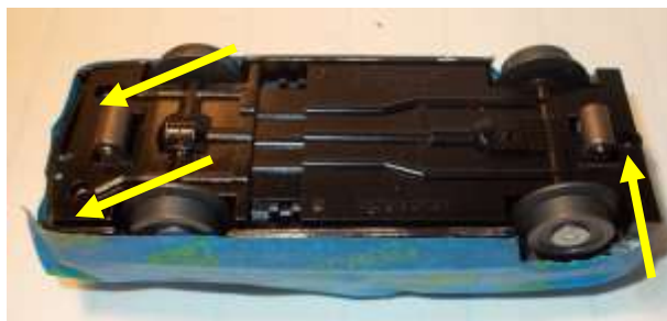
Figure 10: Blue painters tape protects the body during cutting and other operations.
