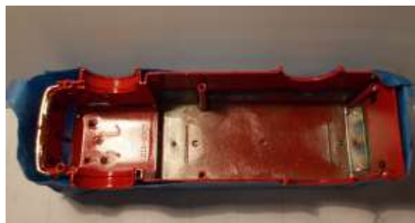
Figure 4: The interior is remarkably free of towers or metal ribs that could get in the way of the chassis.
