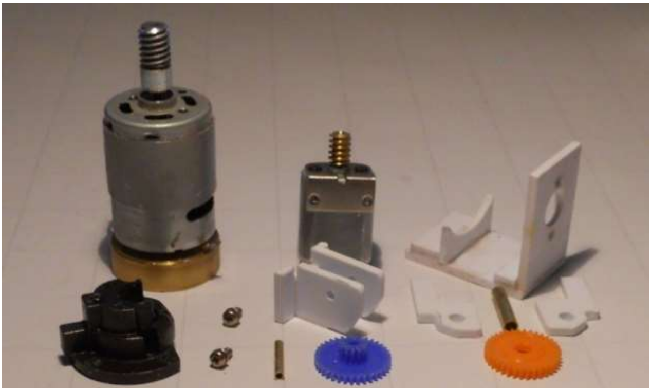
Figure 22: The motor (upper left) can be found in full-size diesels from MTH, Lionel, and K-Line and other manufacturers. This one came from a broken MTH Veranda Turbine. Black casting in the front of motor is original motor mount bracket. The stock 'Streets motor is shown to in the middle back. Blue and orange gears are from Tamiya. Other parts were fabricated or purchased.
