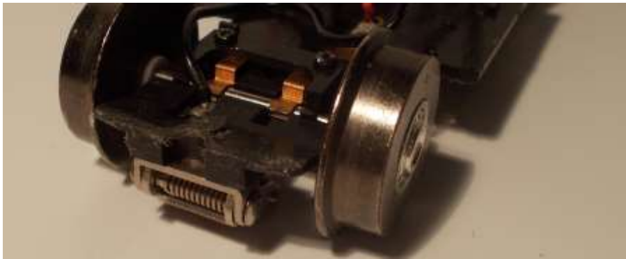
Figure 22: Front post removed and edge trimmed flat.
