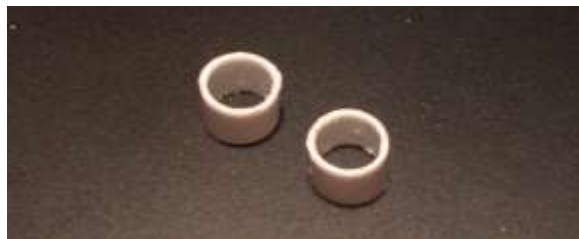
Figure 28: Spacers are made to position back of cab level with front.
