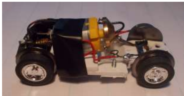
Figure 13: School bus chassis is so short that even stretched by 10 mm it still looks short. It has been upgraded with an oversize flywheel motor as described in Chapter 6.
