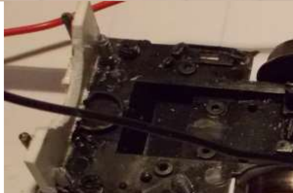
Figure 11: Bare chassis is made from an early K-Line step-van – one with the larger diameter wheels that better match the size needed on a cross-country bus. This chassis also comes with lever-action center rollers that are slightly better than the spring-arm type. White styrene plates at the ends, attached as shown, provide mounting to the unmodified die-cast body, positioning the body at the right ride height to look realistic.
