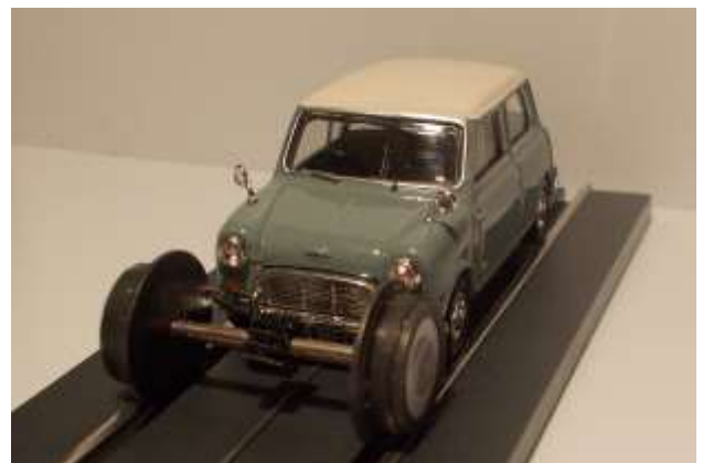
Figure 4: Not going to happen. This 1:43 Mini’s tires fit into the flange grooves! Any O-gauge axle is wider than the car is!
