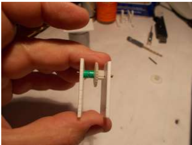
Figure 28: Gearbox partially assembled.
