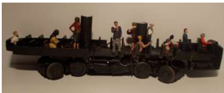
Figure 26: Two-motor sedan-derived center chassis has rigidly fixed axles – both driven. It was strapped to the original interior shortened by the same amount as the body (figures added by author).
