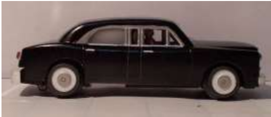
Figure 14: Limosine was made from two bodies. Adjustable chassis was lengthened one notch. First body was cut at B pillar, other body was cut “one notch length” ahead of B-pillar. When glued together they made a body about a scale nine inches longer.
