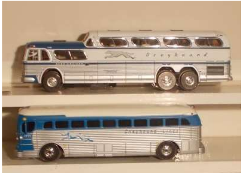
Figure 10: Converted Corgi 1:50 buses from Chapter Seven. Although the Scenicruiser (top) has a wheelbase slightly longer than its sibling, its swivel truck means it runs through curves much easier than the shorter two-axle bus. It needed no additional weight for traction. The lower, two-axle bus, having a smaller body, was about an ounce lighter but required four ounces of additional weight to give it enough traction to run smoothly through curves.
