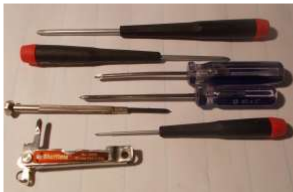
Figure 4: A set of fine Philips screwdrivers is a necessity. Some projects require three or four sizes from 0000 to 1. Other drivers including flat and triangle-heads may be needed for die-cast models.
