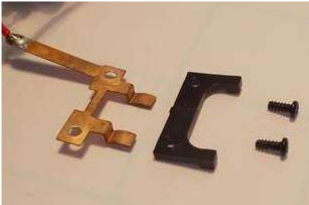
Figure 22: Front-axle contact brush and the plate that holds it and the front axle in place.
