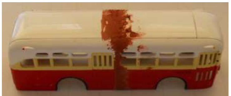
Figure 7: On the outside, Bondo glazing putty is used to fill seams, and allowed to harden. for 24
