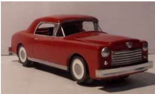
Figure 16: Sport coupe. B pillar was removed, door seams were filled and scribed for a two-door. The A pillars were removed and replaced with new pillars farther back and slanted to form a wrap-around windshield (stock clear front windows are still used). Rear 3/8 inch of roof were removed, trimmed, and glued back in at a sloping angle. Gaps and scratches were filled and sanded, and the body repainted, etc.
