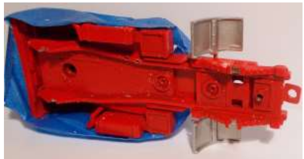
Figure 24: Tractor is wrapped in protective tape. Axle mounts are filed down to shiny metal and so axles fit well.
