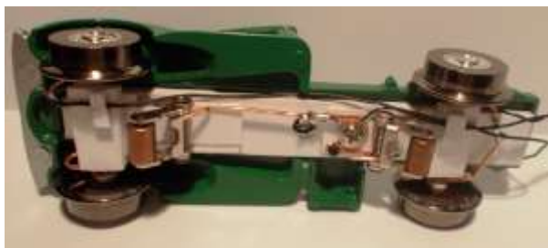
Figure 19: Copper wire is used to make “pickup fingers” for axles and center pickups and wires soldered to them.
