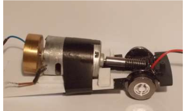
Figure 34: Motor mounted in cradle.
