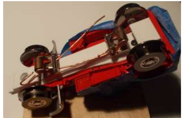
Figure 29: The two center pickups have been installed (Step 6). Copper "picture hanging wire" is used for pickup fingers for both. That on the right has been pulled through but on the driver's side is about to be.
