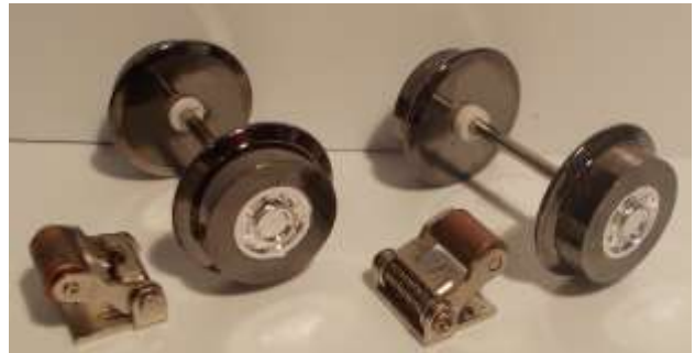
Figure 23: Axles and center pickups from one WBB panel van.
