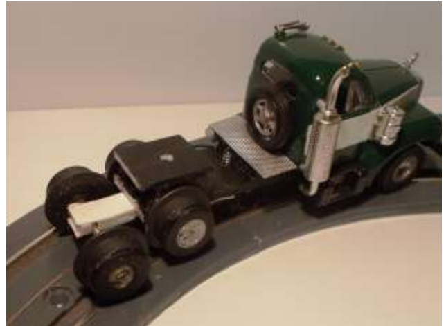
Figure 62: The tractor's third axle stays perpendicular to the chassis axis but can slide sideways in curves. It looks a bit strange as it does, but works well and allows tight back-to-back spacing of the two axles.
