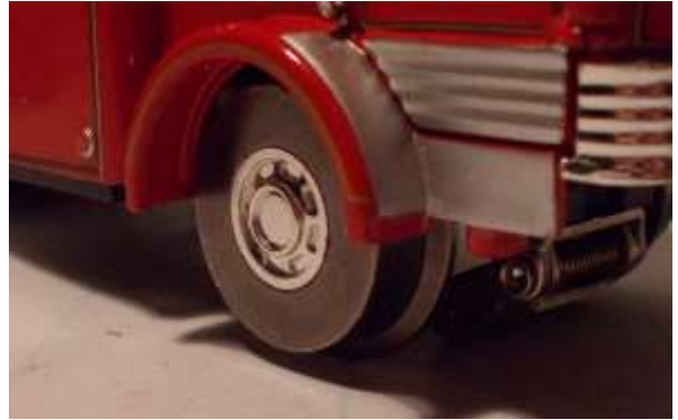
Figure 8: Front wheel wells are 5mm wider than the outer edges of the tires.
