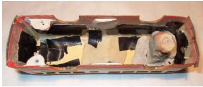
Figure 8: Repair putty is used to make three mounting towers for the chassis,
