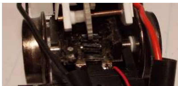
Figure 13: Power unit positioned properly: the secondary gear is centered on the rear axle gear and perpendicular to it.
