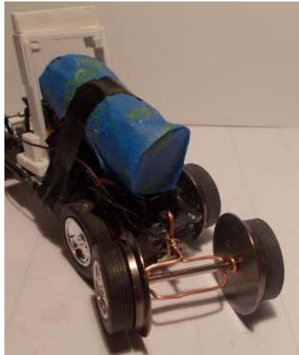
Figure 17: The third axle may look a bit crude but it works perfectly . Thin copper wire bends easily to make the frame and assures excellent electrical conductivity to the wheels: Only their weight keeps them on the rails, but that is sufficient.
