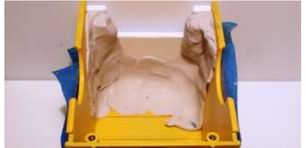
Figure 33: Repair putty is mushed around the junction of panel and body to hold it in place. It is made thick near the sides to provide room for mounting screws.
