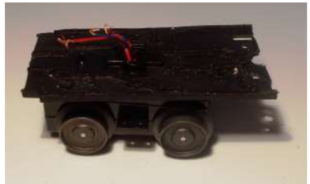
Figure 51: The truck from the trolley was removed and tested. The chassis was trimmed as described in text shown here.
