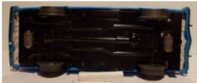
Figure 21: Repair putty at both ends of the Dodge body forms attachments for the shortened but unmodified chassis.
