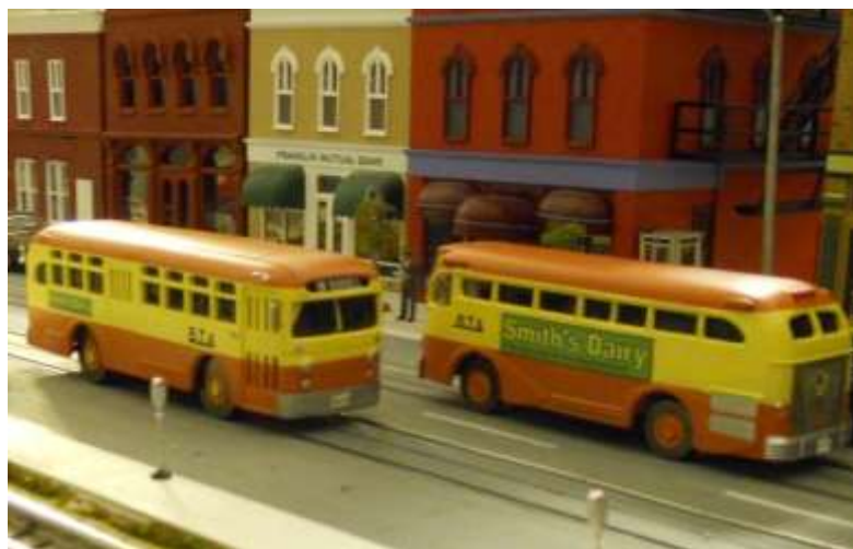
Figure 5: Wheelbase of these two 1:50 Corgi buses was shortened by 1 \frac{9}{16} inches, so they match the wheelbase of the step-van, on which chassis they are mounted. In many cities, real versions of city bus models were manufactured in shortened versions like this for much the same reason as done here: so they could negotiate tight city corners.
