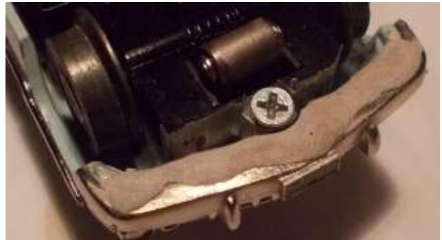
Figure 37: Detail of front of the DeSoto's chassis shows a type of trimming necessary with many models that have a short front overhang. The front of the chassis is trimmed off but a small tube of metal about 2 mm thick is retained around the mounting hole.
