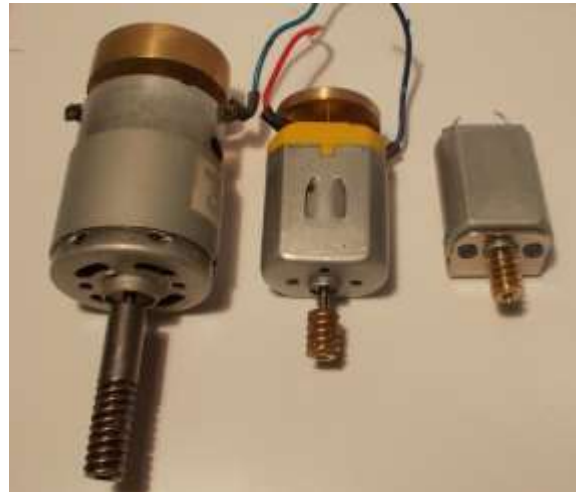
Figure 6: Right, a standard ‘Streets motor’. Middle, a motor with about twice the power and a flywheel, used in the “Modest Motor Upgrade” in Chapter 6. Left, “Immodest Motor Upgrade” is a motor from MTH and Lionel diesels, which the author uses to repower buses and trucks. Part numbers and details are given in Chapter 6. True?
