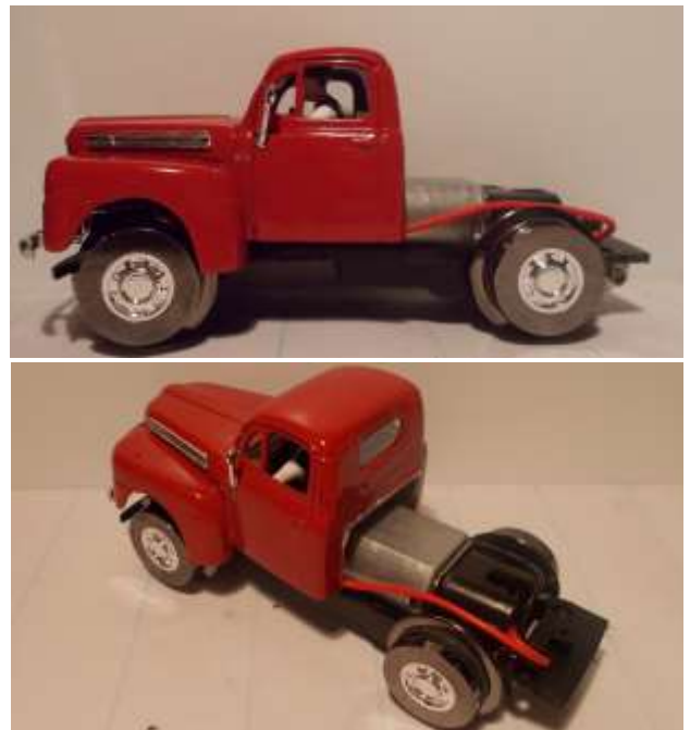
Figure 8: Cab mounted on chassis. The author has trimmed the portion of the chassis behind the rear wheels narrower (compare to Figures 5 and 6).
