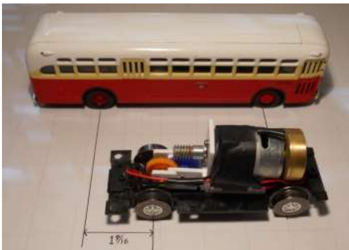
Figure 2: Corgi 1:50 GM 4510 bus has a wheelbase 1 9/16 inches longer than the 'Streets step van chassis
