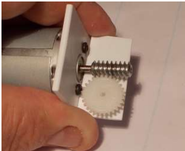
Figure 27: Find two gears as described in text, and a metal rod (not shown) to make gear shafts on which they can rotate.
