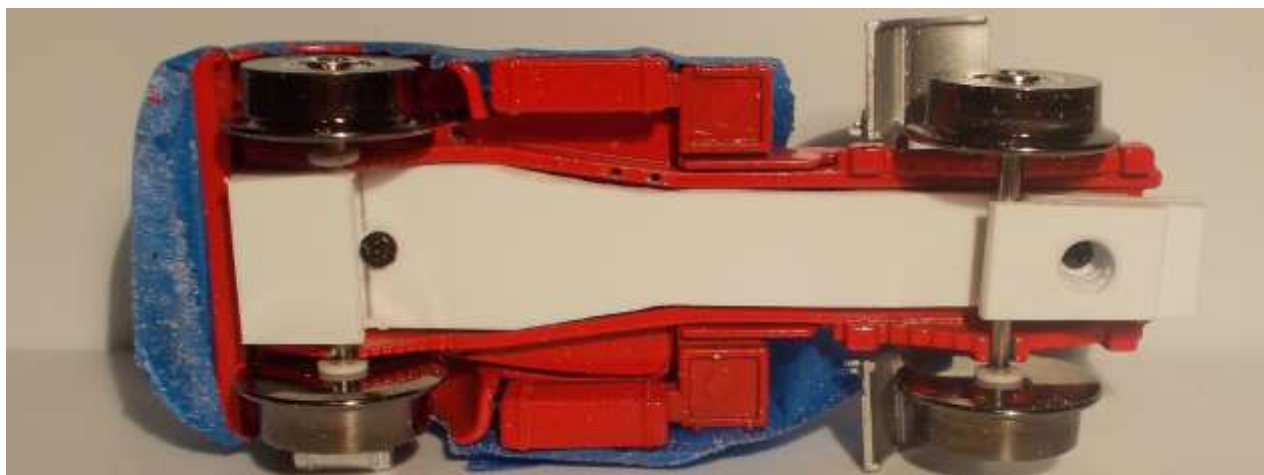
Figure 27: Chassis insert installed and retaining the axles.
