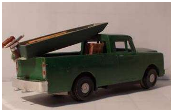
Figure 17: Horizontal cut was made through entire truck 3/16 inch above top of wheel wells, and a 1/8 inch thick styrene sheet inserted and body glued together (raises body height by a scale 6 inches, and forms pickup bed “floor”). Windshield was repositioned more vertically. Scratches were filled, sanded, and truck painted.
