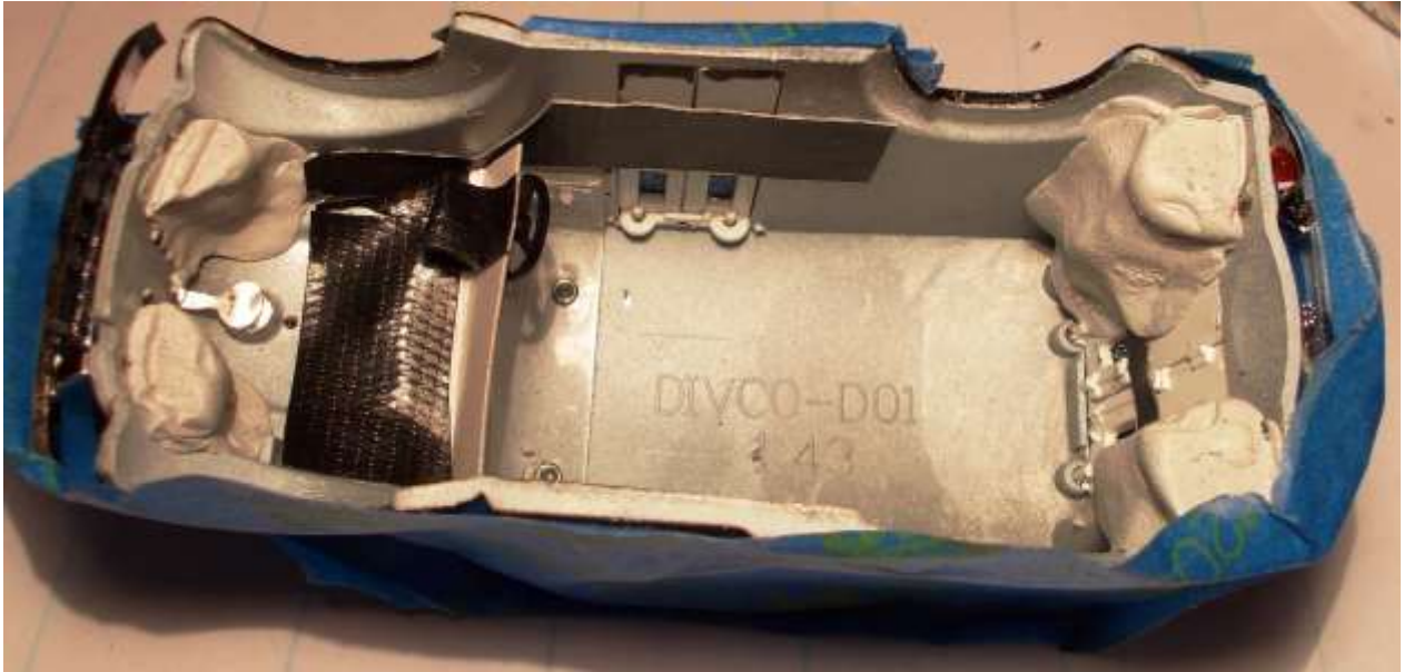
Figure 32: Four mounting-positioning towers were made from Repair Putty. Gorilla Tape was used to fasten doors somewhat better during modification (the 'Streets chassis will secure them firmly in place once inserted in the body). Dashboard is just taped in place.
