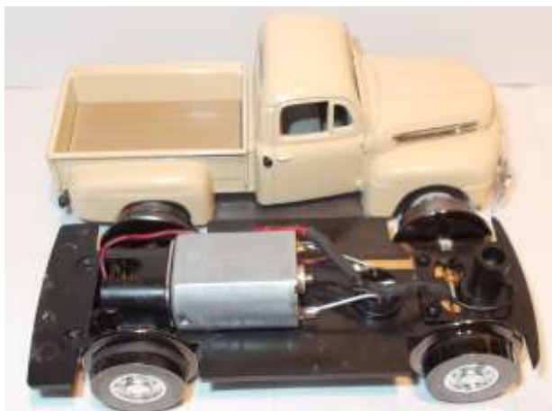
Figure 44: A sedan chassis will not fit in the Road Signature Ford F-1, but a plastic panel van chassis has just the right wheelbase and plastic is easy to work.
