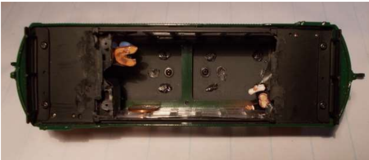
Figure 22: Underside of trolley was cut as shown. See text for details.
