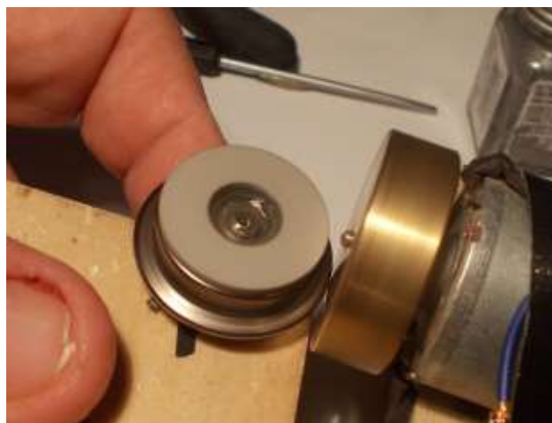
Figure 12: Unpowered axles or loose axles are pressed against the spinning flywheel to spin them. While they spin, a paintbrush is then held against them spread paint circularly.
