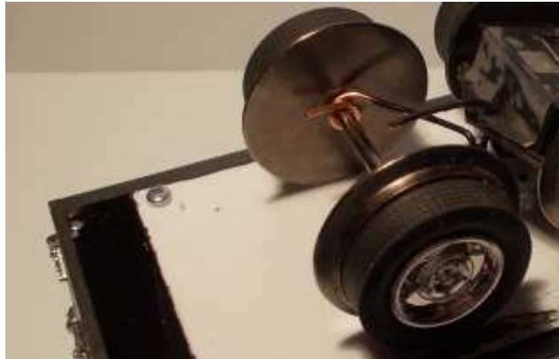
Figure 47: Second axle is a swinging trailer-axle that was simply hooked into a small hole drilled in the back of the school bus chassis.
