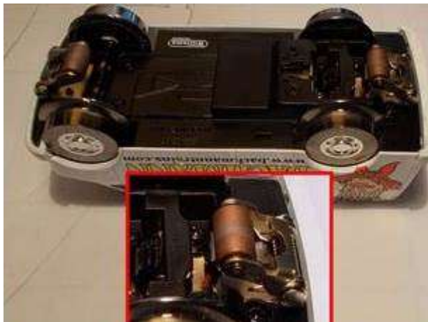
Figure 26: When it began producing the new E-Z Street product line, Williams by Bachman replaced the spring-arm rollers (Figure 7) on the plastic chassis with small lever action rollers shown here. They work much better, in the author's opinion justifying the slightly higher price Bachman charges for their versions.
