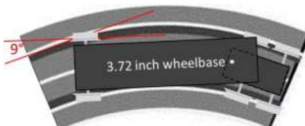
Figure 4: A two-axle swivel truck on a bus (Scenicruiser example in Chapter 8) or truck reduces friction tremendously. In addition, moving the pivot point (white dot) forward reduces the angle of attack for the front axle, further cutting friction and permitting a still-longer wheelbase before flange binding occurs.
