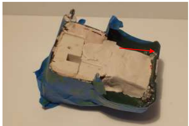
Figure 25: Cab is covered with painter's tape. Loctite repair putty is pushed into every nook and around the interior, filling the cab flat to the level of the lower edge of the cab: note the 1/16-inch high lip left at the front by doing this. Wheel wells are left empty so there is room for wheels.
