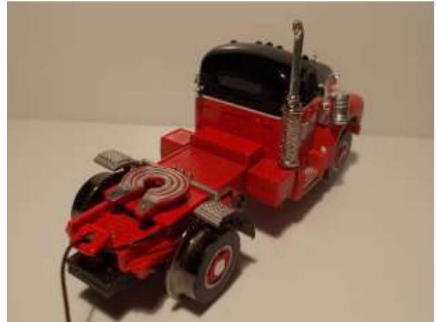
Figure 40: Tractor's trailer mounting tongue is cleaned of paint to improve electrical connectivity through it.
