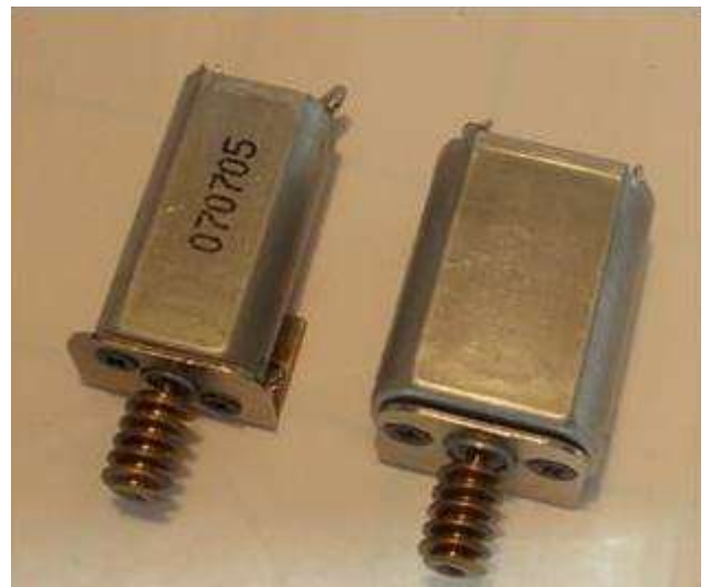
Figure 23: The vintage truck uses the motor on the left; all others use the motor on the right. Both types have a press-fit brass worm gear on the front shaft, no flywheel, and a mounting plate held to the front face by two machine screws. The larger one has a motor body exactly 1 inch long.
