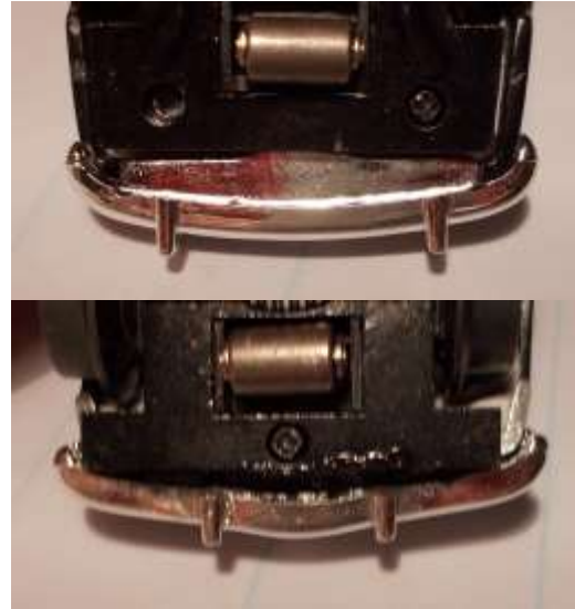
Figure 15: The bumpers have to be trimmed as shown here, and then glued onto the body. Compare to Figure 3.
