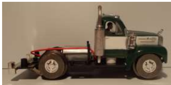
Figure 29: Cab mounted on chassis. The spacers have been put in place and a screw inserted through each into the bottom of the cab putty/interior floor.
