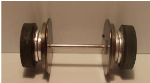
Figure 8: Bus tires have to be glued in place, and new wheel hubs made inside each tire, as shown later, so the bus axle gains width to match larger 1:43 model truck widths.
