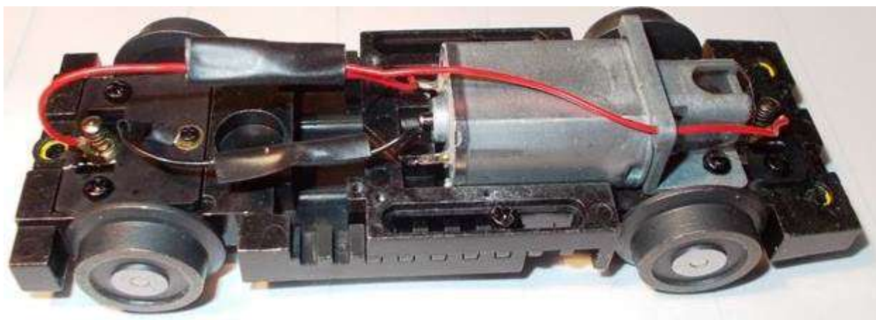
Figure 34: WBB sedan with the re-wiring completed. The rectifier has been removed, the wires soldered as indicated in the text, and the junctions taped. The vehicle will now go forward when positive DC polarity (positive on the middle rail) is fed to it, and backwards when that polarity is reversed.
