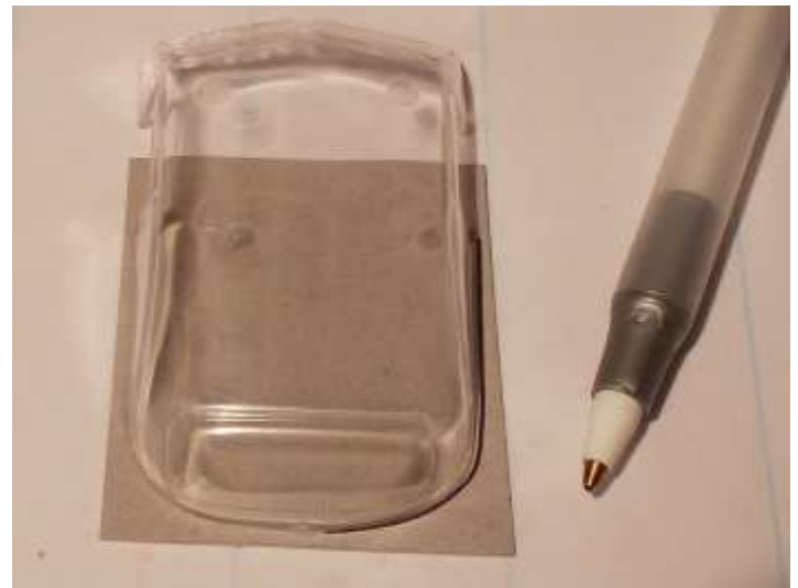
Figure 14 Trace the window piece from the B pillar location back to make the rear interior cover.
