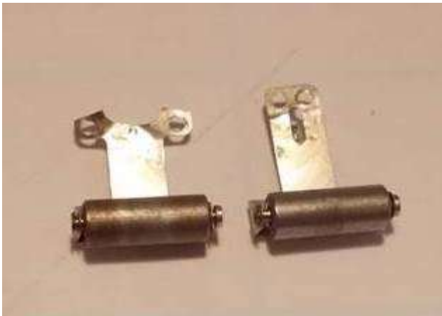
Figure 25: Although similar in construction the front and rear rollers on plastic chassis are of two types, as shown.
