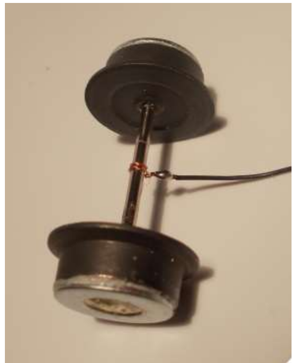
Figure 54: Homemade outer-rail pickup from the axle works very well.
