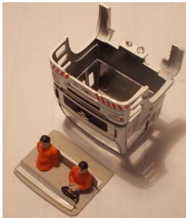
Figure 14: New interior is thin cardboard cut to fit snugly in the cab up against the lower edge of the plastic window piece inside the cab. Cardboard dash, two figures, and a steering wheel complete the interior.
