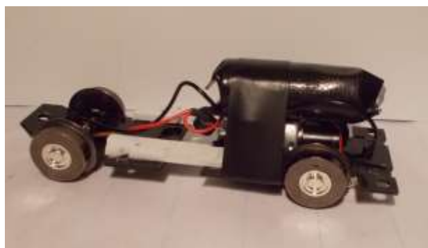
Figure 9: This step-van chassis was lengthened about one inch (see Chapter 7's Corgi Mack fire-truck example). Although the new die-cast body weighed a bit more than the original 'Streets body, a roll of thirty-two pennies (three additional ounces) was mounted atop the motor. This provided sufficient traction without adding so much weight it would overwhelm the stock motor, and while the power is while barely sufficient, in this case it is sufficient.
