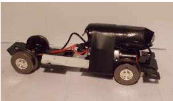
Figure 9: A roll of thirty-two pennies (3.0 oz.) was taped above the motor: it just clears the roof of the die-cast body, but fits. This improved traction and speed through curves nicely.
