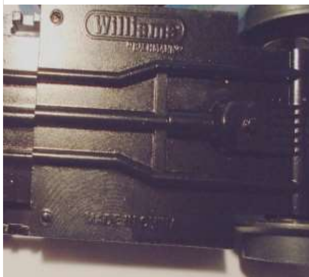
Figure 11: The author deliberately touched the bottom of the chassis here to demonstrate. Nothing but sandpaper is going to remove this epoxy fingerprint. Wash hands after using the putty!
