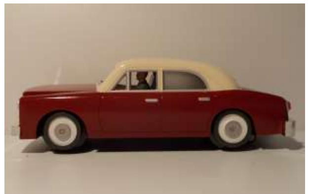
Figure 15: The sedan is 117 mm long by 43 mm wide by 37 mm high. The wheelbase is 69 mm, adjustable by +/- 10 mm. It weighs just 7 oz. Author added driver figure.
