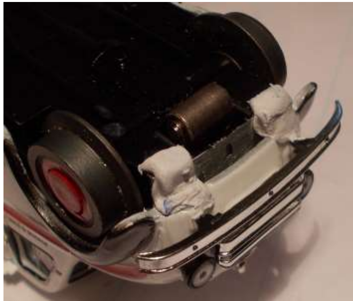
Figure 34: Once the chassis is mounted and the screws in the rear are screwed down, repair putty is used at the front to make these two small hook-tabs that hold the front in place.
