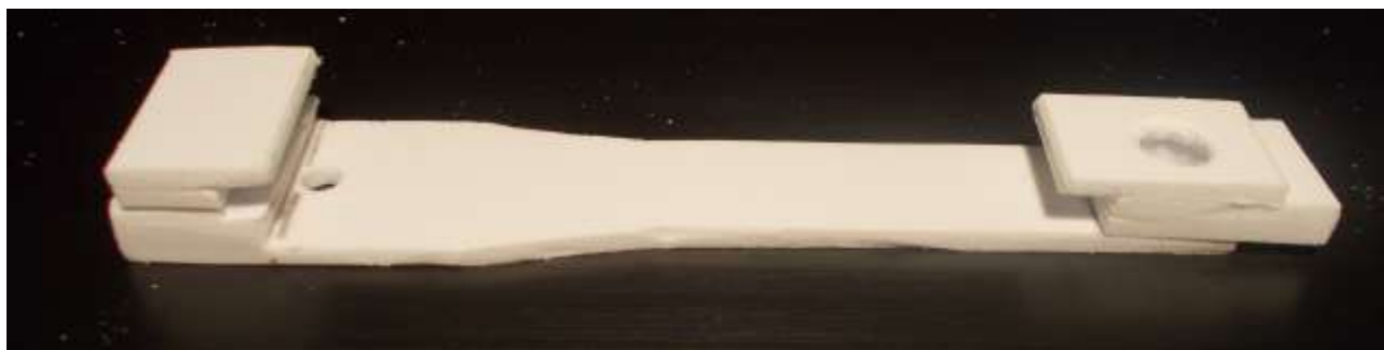
Figure 26: Chassis insert is built up to make the front and rear axle retainer towers.
