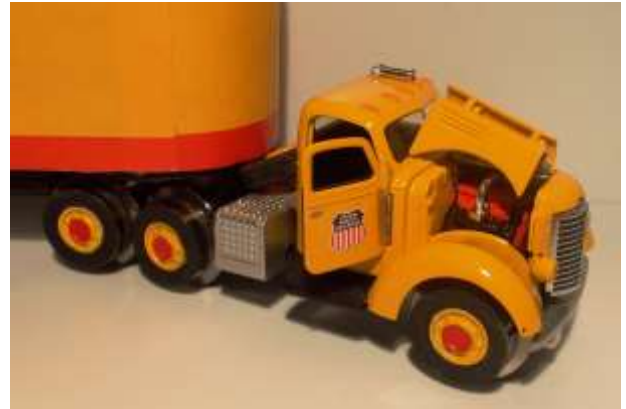
Figure 15: Motor-less conversion of a 1:50 SpecCast International KB tractor allowed a prototypically correct trailer mount height and retention of the original model's cab unmodified, including its opening doors and hood and model engine.
