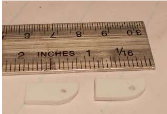
Figure 32: Two rectangular styrene pieces made for the secondary-gear frame arms.
