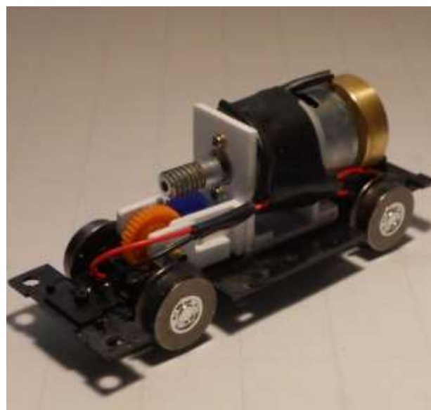
Figure 3: Step van chassis with large-motor power unit (see last section of Chapter 6).
