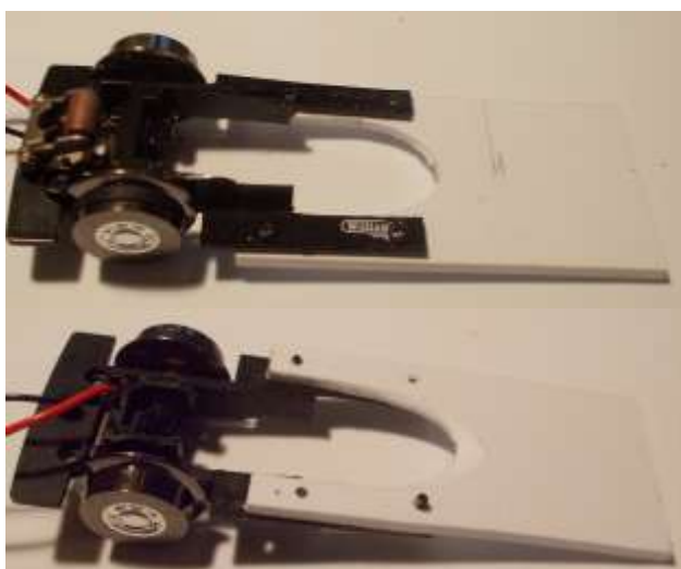
Figure 32: Two views of the panel-van chassis with its rear axle, as cut and trimmed, and the “motor cradle” screwed to it. Note the parabola’s edge is filed at an angle to maximize contact space/support.
