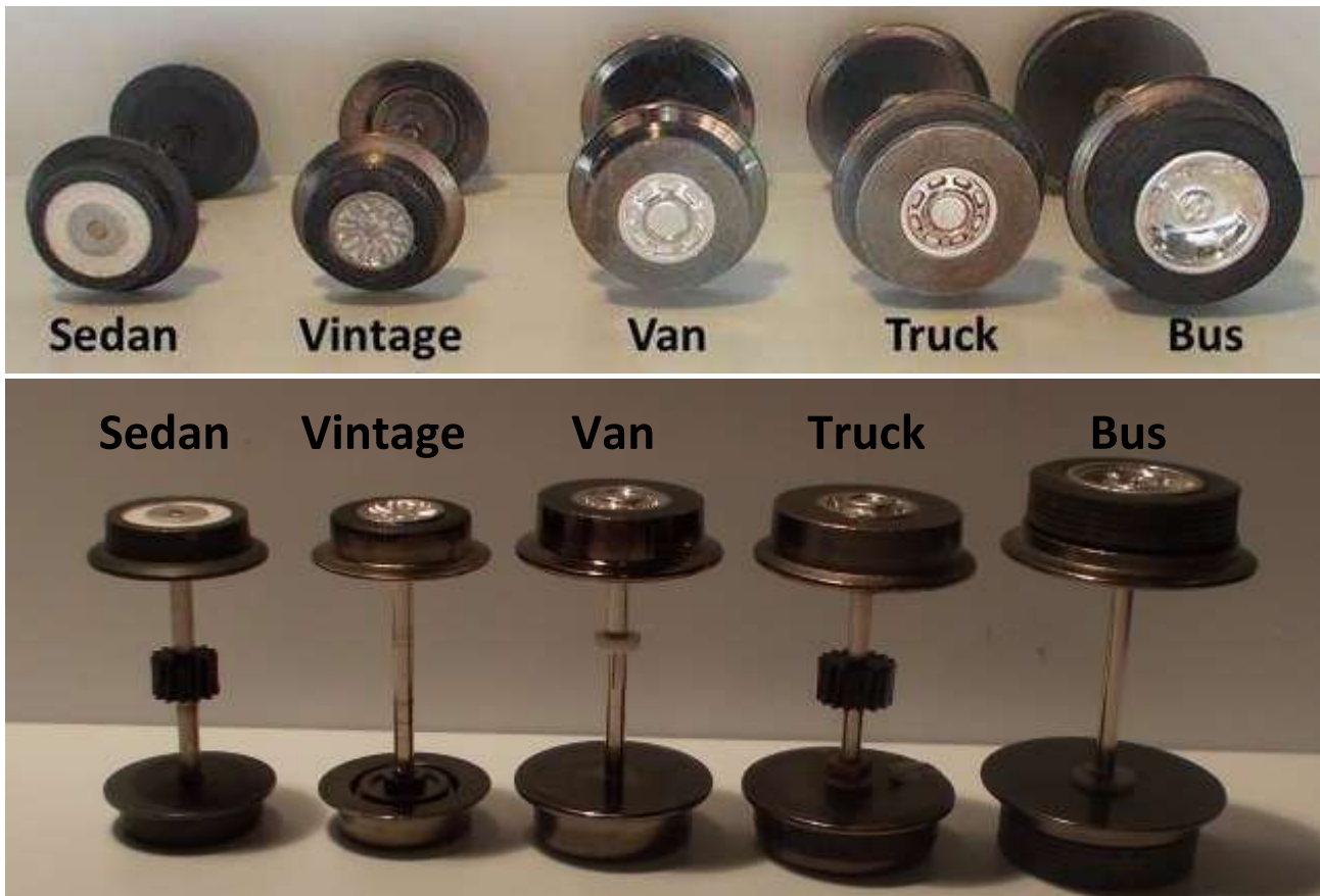
Figure 1: Wheels from the five types of 'Streets chassis. They vary in diameter by nearly two to one and vary in width across the wheel outer edges by a scale eighteen inches.
