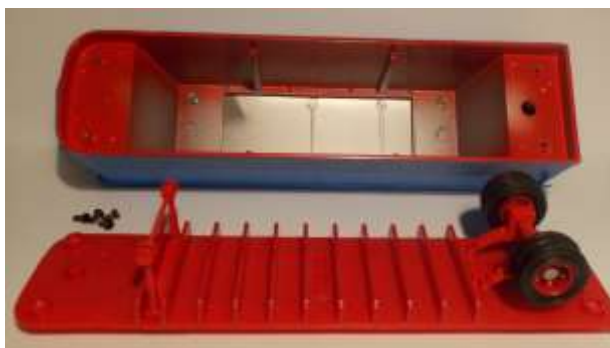
Figure 31: Trailer disassembles by removing four screws for underneath.
