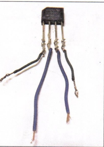
I used a 400V single-phase bridge rectifier for this project.
