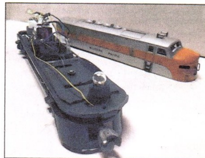
Lionel's O gauge diesel models from the early modern era tend to have more space for the installation of a rectifier than did its steam locomotives.
